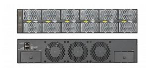
NETGEAR M4300-96X (empty switch) is a NETGEAR modular managed switch chassis used for large AV over IP deployments. It can be populated with module units in increments of 8 10GBASE-T, 8 10GBASE-X (fiber SFP+) ports or 2 QSFP+ ports. NOTE: Only the first 6 slots deliver PoE power to the 10GBASE-T cards, enabling a maximum of 48 PoE+ ports per switch. APS1200W is the preferred PSU for PoE power
